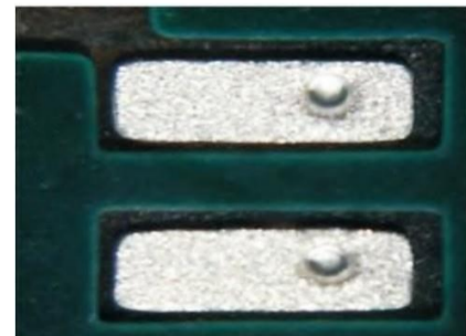
Blind hole fully covered by Tin layer
