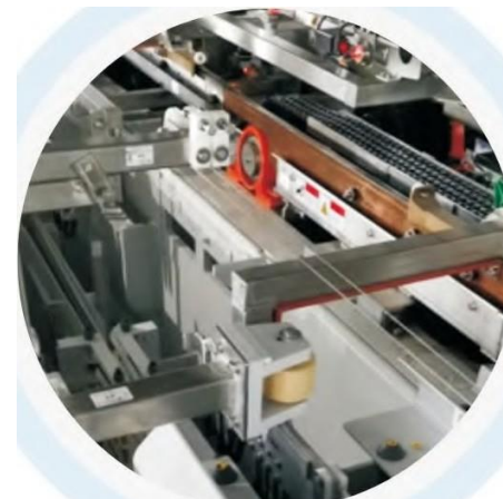
Copper tank is equipped with steel wire rope. Alarm starts when flight bar jiggles
